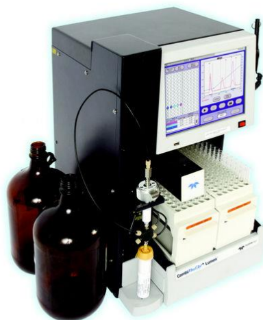
Figure 1. Liquid chromatograph Teledyne Isco Combi Flash RF+. 6
