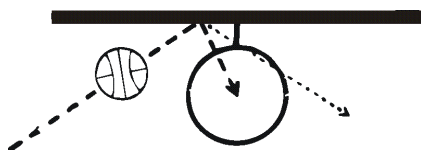
Figure 62: Rebound angle of a ball with zero spin from the basketball board – top view (Dobry 1963).
